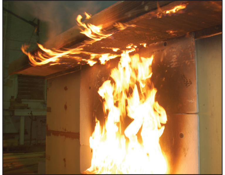
Direct flame on siding burns into the eaves and roof. Photo by Institute for Business and Safety Research Center.
