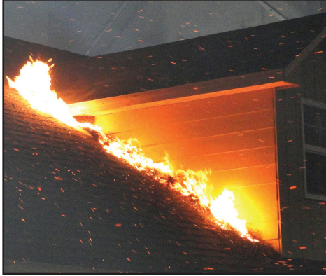
Leaves and needles burning along roof edge with dormer. Photo by Institute for Business and Safety Research Center.
