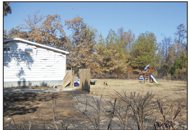
This home escaped the flames when firefighters knocked down the burning fence that would have led flames to the home. Notice the burn marks on the fence.
