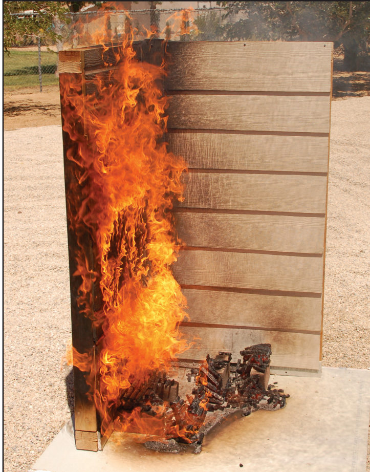
This photo shows the difference between combustiblesiding (left) and fiber cement siding (right) when exposed to the same direct flame source. Photo by Institute for Business and Safety Research Center.
